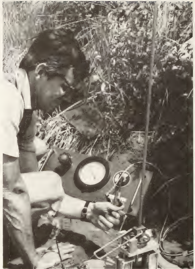
Figure 16. — Borehole, direct shear test in progress in shallow, coarse-textured soil developed on granitic rocks of the Idaho batholith. Pine Creek study area, Boise National Forest.
